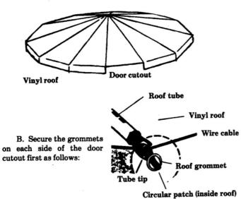
Stand outside the screenhouse and grasp material and grommet with both hands, exposing underside of grommet and circular patch, as shown below. Be sure patch is fully spread. Pressing both thumbs agains screenhouse frame for leverage, pull edge of vinyl toward you and secure grommet to tube tip.
