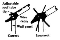
winds. The cable must be located fully in the eye of the plain tube tip.
