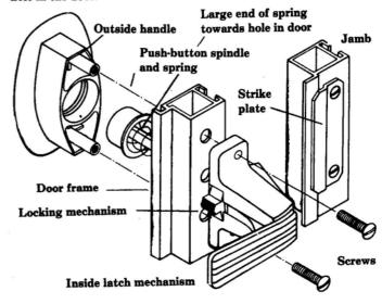
C. Insert assembly through drilled holes from the outside of door. Position inside latch mechanism over the holes on inside of door, guiding end of push-button spindle into rectangular slot in latch. Fasten with the two machine screws provided.
