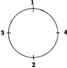
The remaining tubes should then be installed directly opposite each other, following the same procedure for each tube.
