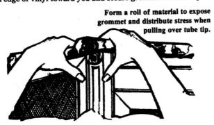
Next, fasten the two grommets on the vinyl roof section directly opposite door. Proceed to fasten balance of grommets over tips. Always fasten grommets on side opposite to the one previously secured.
