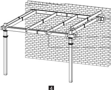
Finally, adjust the main support beam and rafters ensuring the overhang past the column is equal. Using 4" (102mm) screws, lock the main support beams and rafters into position inside the posts by driving in 4 screws from the front and back each, and 2 screws from the sides of each column.
