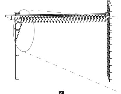
If your area experiences heavy snow, make sure to keep the louvers in the **OPEN** position. The accumulation of snow will cause the louvers to buckle and collapse.
